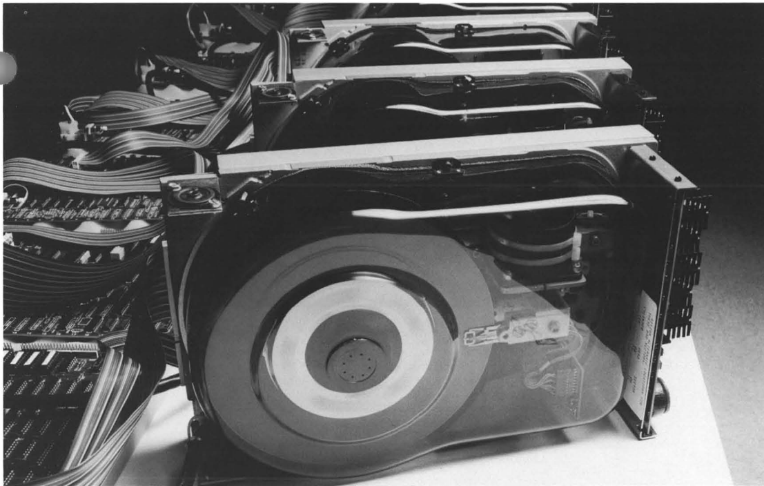
Production units of the 101 8-inch mini disc drive are undergoing final test in the Company's 100,000 square-foot plant in San Jose, California.
